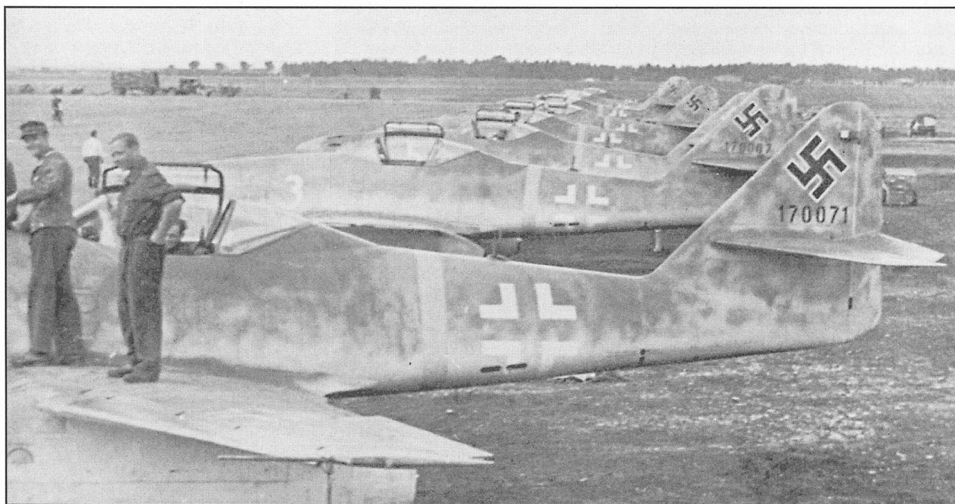
Eight Me 262s of Erprobungskommando 262 lined up at Lager-Lechfeld. In addition of yellow numbers painted on the nose, EKdo 262 used a yellow band painted around the fuselage forward of the national cross. The Werk-Nr. is painted in black just above the horizontal stabilizer. (Air Force Museum Collection)
