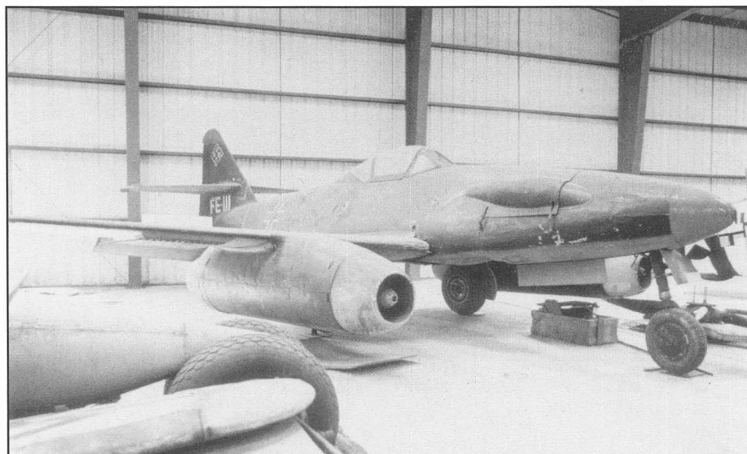
FE-111 was an Me 262A-1a/U3 interim reconnaissance version captured by the Americans. This aircraft was initially named 'Dennis' and is now in the National Air and Space Museum. The bulge required to cover the camera installation is clearly visible. This particular aircraft does not appear to have been fitted with the single 30mm cannon installed on some. (Air Force Museum Collection)
