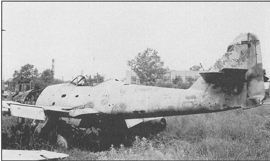
Another Me 262A-1a damaged from Allied bomb attacks. The port engine has been removed, perhaps to install on a more serviceable aircraft. (Air Force Museum Collection)
