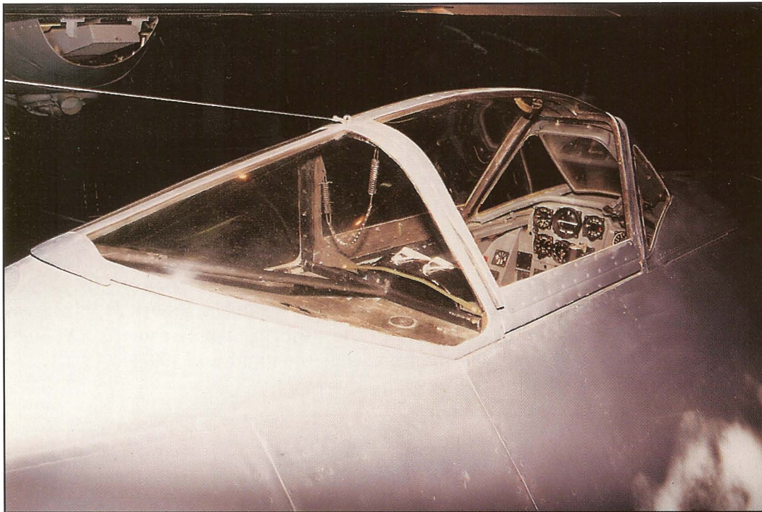
The wire aerial for the short wave radio set was stretched between the top of the rear canopy bow and the top of the vertical stabilizer. The thickness of the front windscreen armor can be seen here. (Dennis R. Jenkins)
