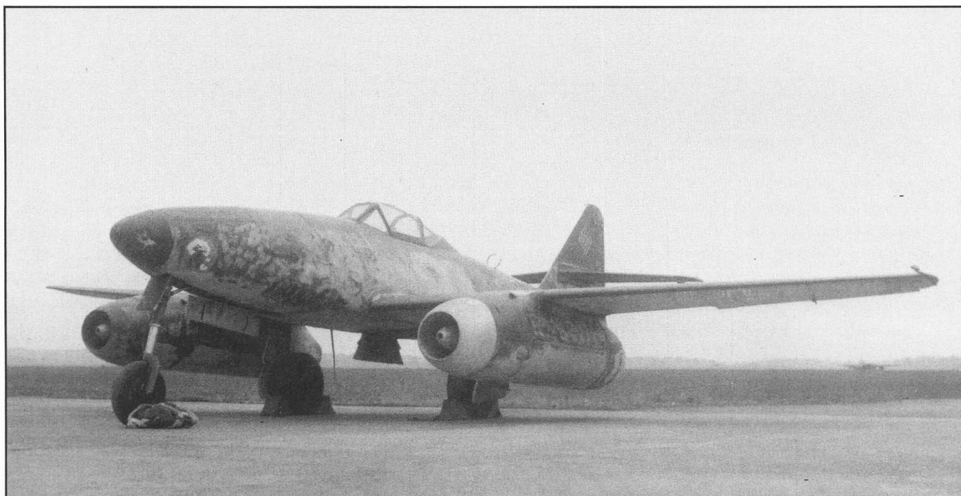
This Me 262A-1a was also captured by the Americans and numbered FE-110. The inlet of the port nacelle has apparently been replaced and a Watson's Whizzers emblem is clearly visible on the nose. (Jay Miller Collection)
