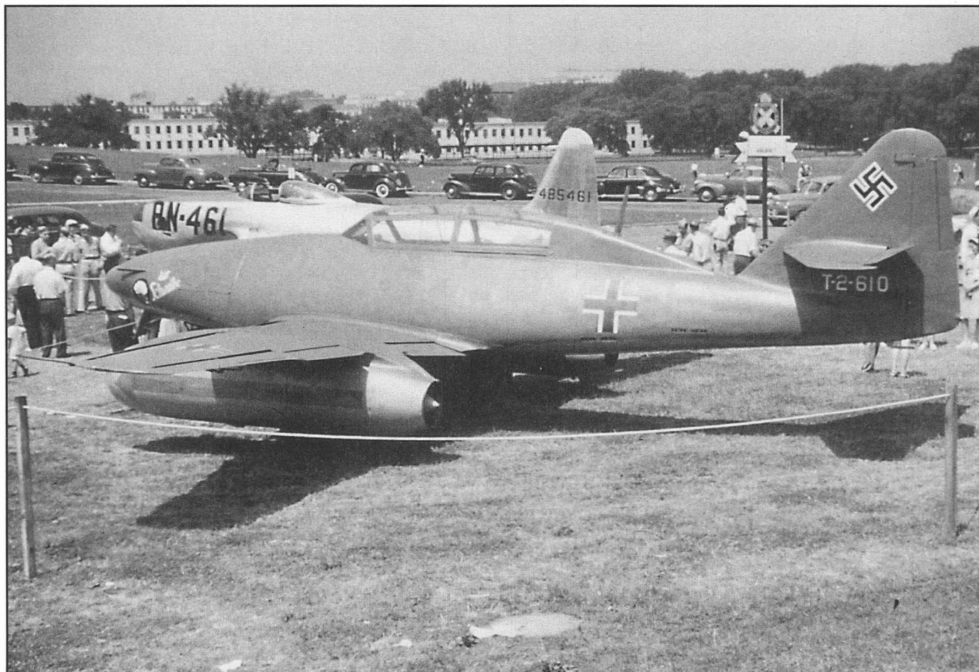
Me 262B-1a/U1 (Werk-Nr. 110306) on display in Washington D.C. on 1 August 1946. At this point the aircraft was still flyable although the Hirschgeweih radar array had been removed from the nose, and most probably the radar equipment itself. This is the same aircraft as FE-610, the designation simply changing to T2-610. The last reported location of the aircraft was at Cornell University in the early 1950s. (Air Force Museum Collection)
