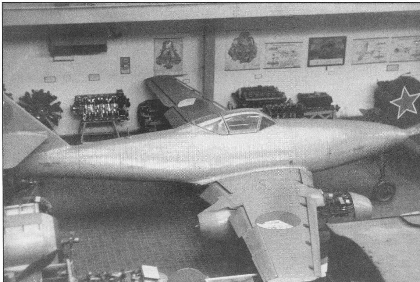
A single-seat Avia S-92 in the VM Aviation and Space Flight Museum in Kbeli. This aircraft was assembled from an uncompleted Me 262A-1a and used Jumo 004B-2 engines. There were initial plans to modify the aircraft with stronger landing gear and BMW 003 engines, but these were overcome by the availability of inexpensive Soviet MiG fighters. (Jay Miller Collection via the Aerospace Education Center)
