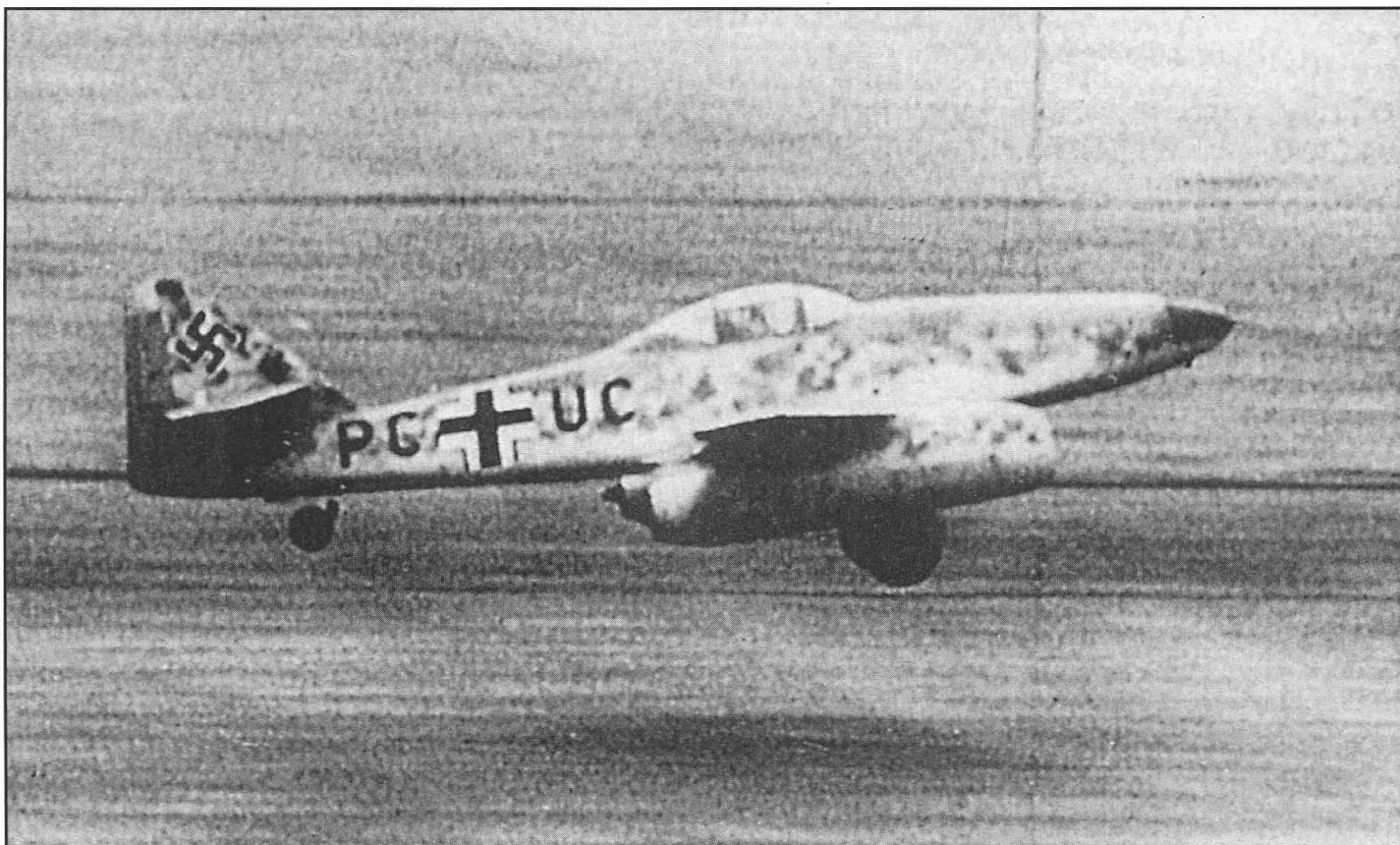
18 July 1942. The third Me 262 prototype takes off for the first time under jet power. Pilot Fritz Wendel was not at all sure the aircraft would lift its tail sufficiently to get airborne, but a brief tap on the brakes proved to be the trick. (Air Force Museum Collection)
