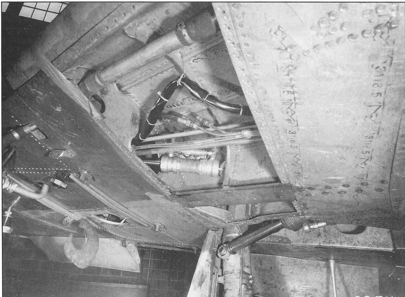
The underside of the wing without the engine nacelle attached. The wingtip is to the left, and the leading edge is at the top. A panel has been removed to allow access to fuel and hydraulic plumbing. (Air Force Museum Collection)
