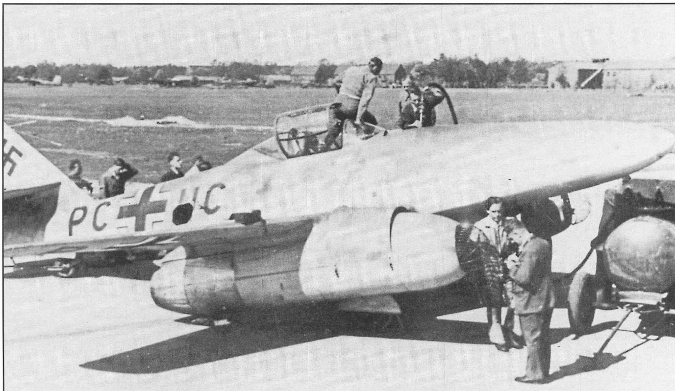
The third prototype is refueled on 18 July 1942 between the two flights made on that day. The screens covering the jet intake is noteworthy. The open panel in the rear fuselage gives access to the push-pull control rods. Paint and markings are fairly typical for the early prototypes. (Air Force Museum Collection)
