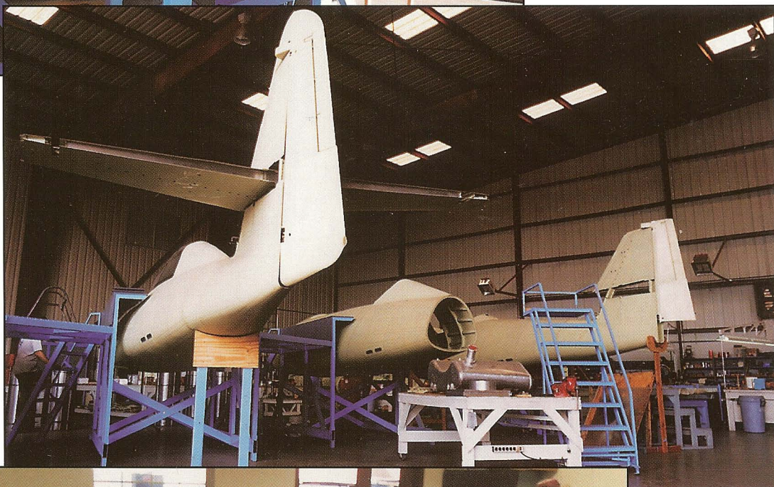
A real Jumo 004B sits in a jig at the Texas Airplane Factory. This engine was used to create forms to cast perfect replicas that will house the General Electric J-85 engines used by Tischler's aircraft. (Jay Miller)
