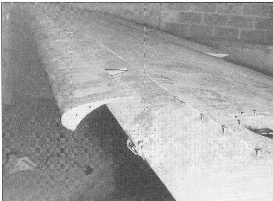
The starboard leading edge slots in the extended position. The engine nacelle is missing. The slots were manufactured from sheet steel since it was readily available and easy to manufacture. (Air Force Museum Collection)
