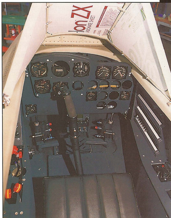
The cockpit of the first Tischler aircraft after it has been installed. The only concession to modern technology (besides the engines) is a small avionics stack on the bottom-center of the main instrument panel where the bomb fusing panel should be. (Jay Miller)
