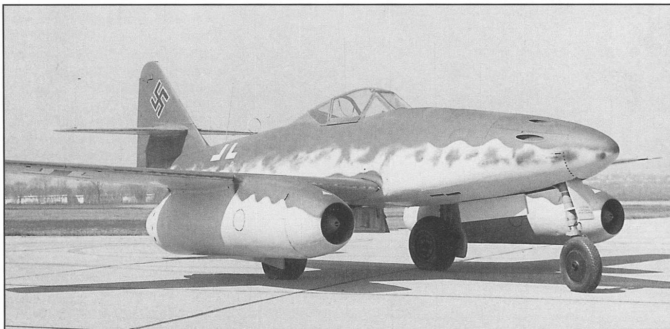
The Air Force Museum's aircraft after restoration. Today this aircraft resides inside the main museum building, well protected from the elements. Most all subassemblies are still with the aircraft, the cockpit is mostly complete, as are the fuel tanks and various radios and other equipment, although the aircraft is not in flyable condition. (Air Force Museum Collection)
