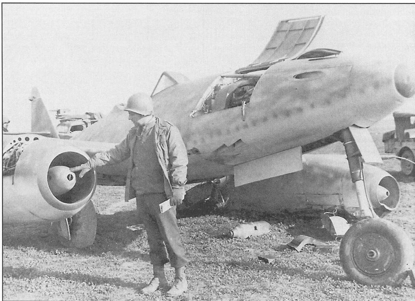
Me 262A-1a Werk-Nr. 500079 (F1+DA) from Stab/KG 76 at Giebelstadt after its capture. The aircraft had apparently suffered minor damage after the collapse of its left main landing gear. The torque-tube that supported the top of the nose section is visible in the access space. (Air Force Museum Collection)
