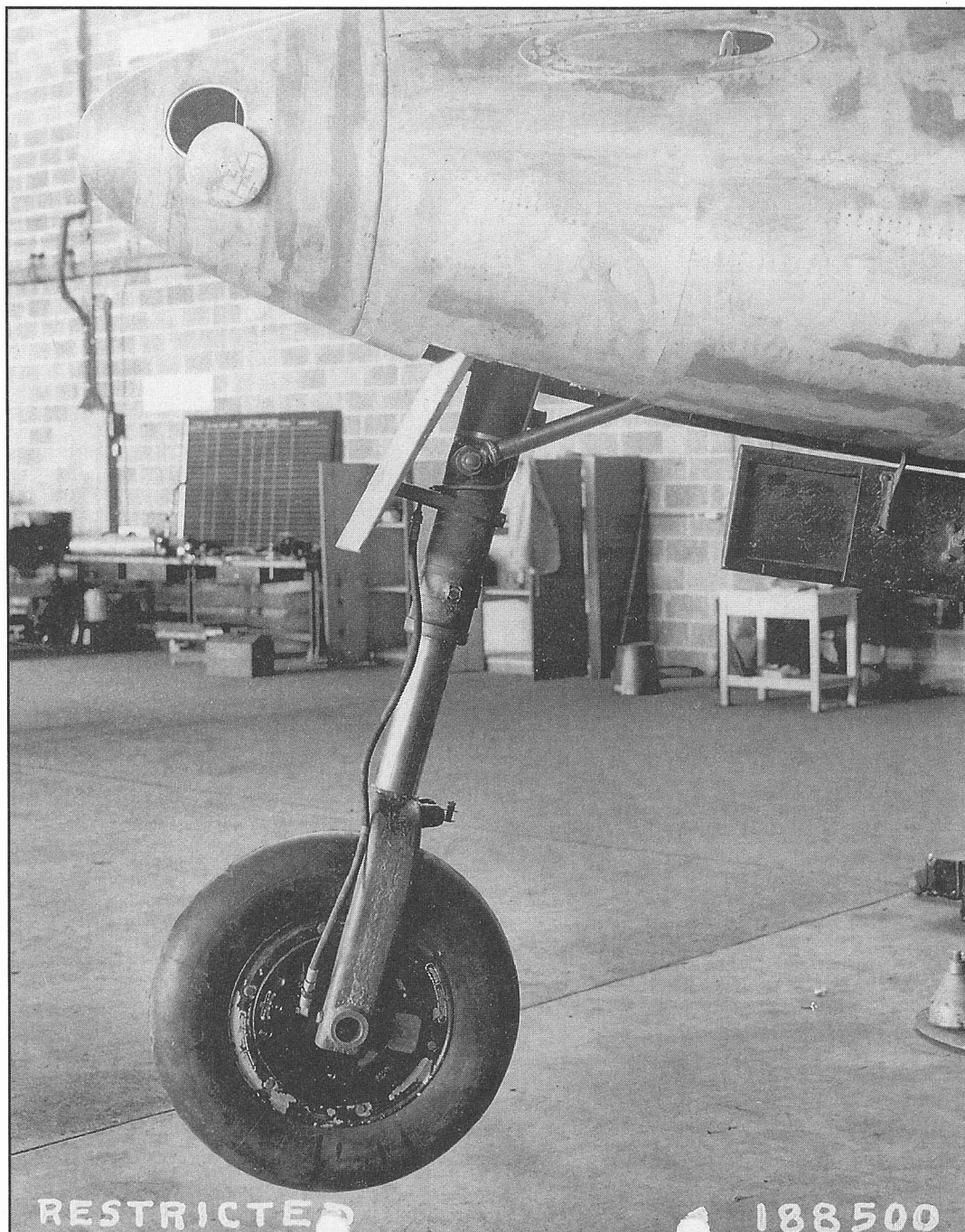
The Me 262 nose gear was a study in simplicity. Unlike the main gear, however, it was equipped with hydraulics for both retraction and extension. The nose gear proved to be a weak point in the Me 262 design, and it frequently collapsed when treated too harshly by inexperienced pilots. (Air Force Museum Collection)
