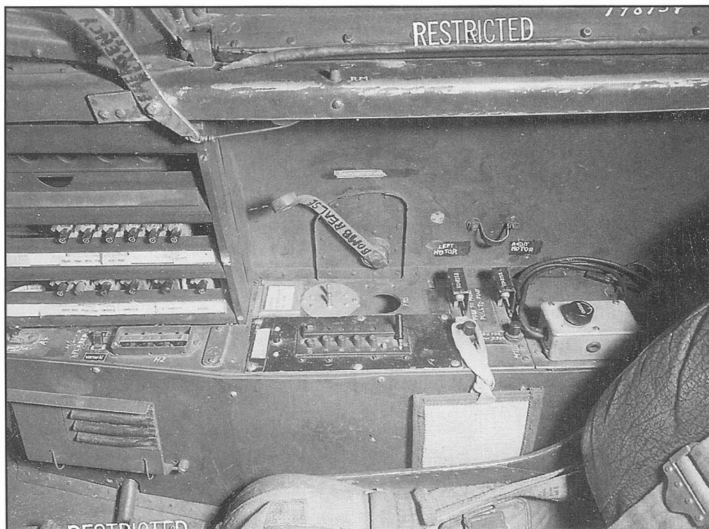
The most prominent feature in this photograph from the December 1945 USAAF foreign equipment report is the 'bomb release' handle on the right-side cockpit wall. This handle has been clearly marked by USAAF personnel. The circuit breaker panel is forward and radio controls are aft. (Air Force Museum Collection)
