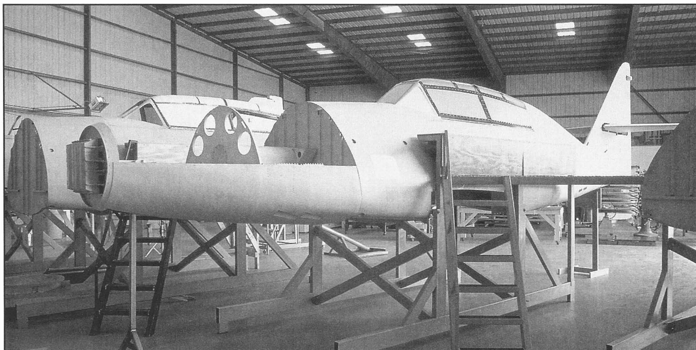
The nose is test fitted to the #3 Tischler airplane. Each fuselage has its own support jigs, allowing production to take place simultaneously. (Dennis R. Jenkins)
