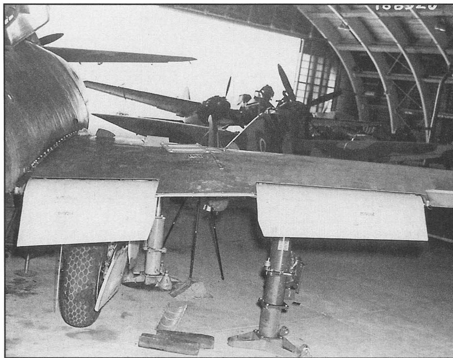
The trailing edge flaps were split around the engine nacelle, which is missing in this photo. The Frise-type ailerons are also missing. This is the Air Force Museum's Me 262A-1a undergoing restoration. (Air Force Museum Collection)
